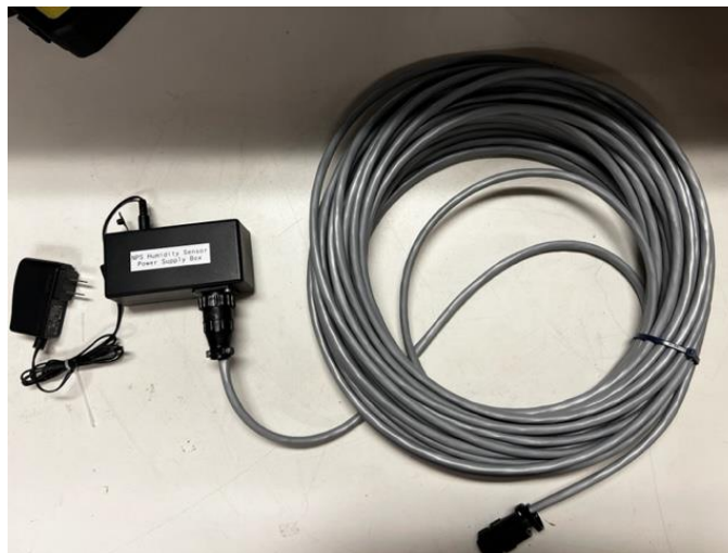
Completed humidity sensor power supply box
